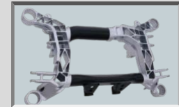
STEEL & ALUMINUM BI-METALLIC STRUCTURES
